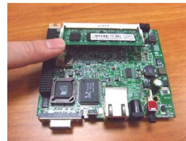
Step 5: Install/Change the DDR2 module
