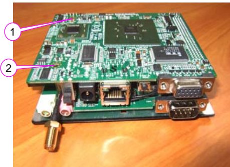
Step 11: Combine two boards (2 screws)
