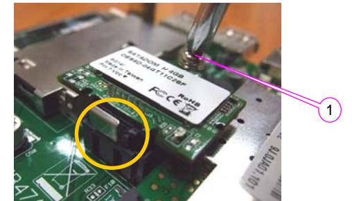
Step 6: Install SATA DOM if necessary (1 screw)
