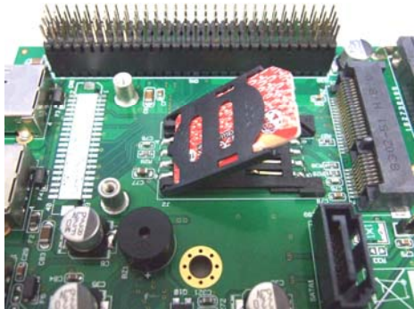
Step 7: Install SIM card if necessary
