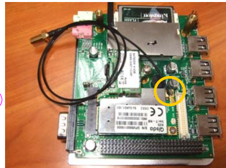
Step 10: Install the Antenna cable
