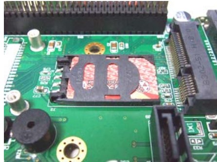
Step 8: Lay the SIM card down as shown
