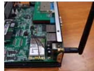
Installing WLAN Antenna (1 of 2)
