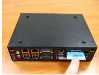
Installing CompactFlash Modules
