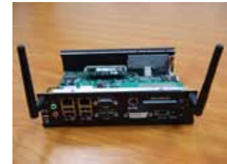
Installing WLAN Antenna (2 of 2, Final)
