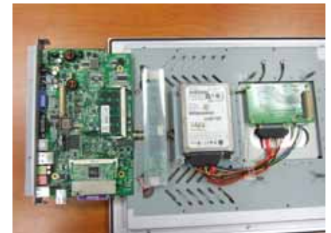
Step 2: Separate the main board from panel carefully and reverse it and put aside.
