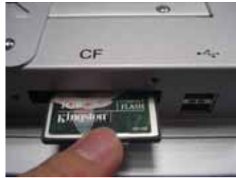
Step 2: Insert CF and close cover
