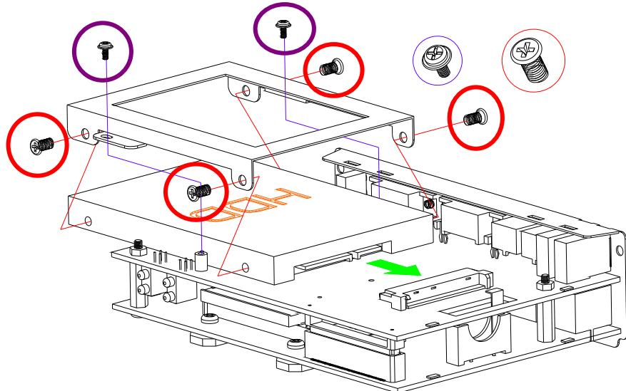
**Note:** Use caution when handling the hard disk to prevent damage to SATA connector as you inserted hard disk. Be careful with the orientation when installing connectors.
