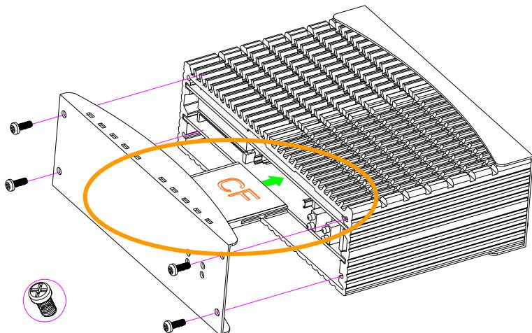
**Note:** The Compact Flash socket supports Compact Flash Modules and Micro Drives.
