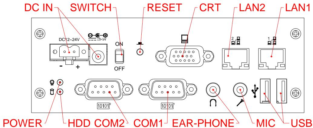
1. A CRT connector is provided for CRT signals
