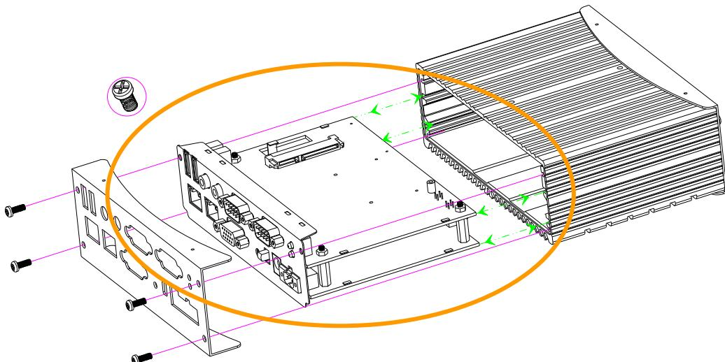
✧ *b1. Installing Hard Disk*
